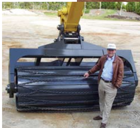
Calvin Thompson, Thompson Grading, developed the Slope Packer as a more cost-effective method for grading contractors to pack slopes and other exposed surfaces on jobsites. His company now has an excavator dedicated specifically to this task.
