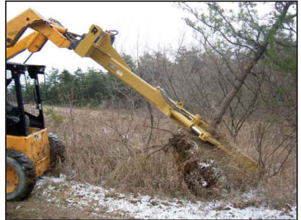
Pull tree out of the ground with your skid steer - roots and all!
