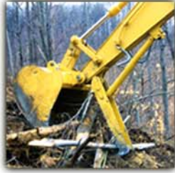
BT-H Hydraulic Bucket Thumbs - in stock for machines weighing 5,001 lbs. to 101,000 lbs.
